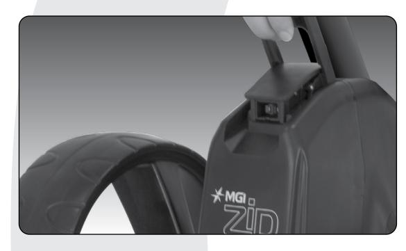
**Step 1:** Disconnect the battery by lifting the battery handle. It can be left on or removed from the Zip Navigator AT.
